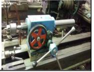
**Fig. 3:** Tail Stock of the Lathe before and after Modification In the proposed method conventional rotating wheel is replaced with gears (gear trains)mechanism which helps the drill bit to move fast by simple rotations as the horizontalmovement of drill bit will be faster comparably(figure.3). Hence with the proposed methodof
